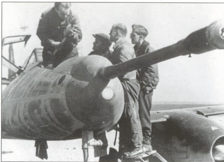
Close-up of the experimental 50 mm Mauser MK 214 cannon installed in the nose of Wk-Nr 111899, the aircraft subsequently flown to Munich-Riem by Willi Herget when he joined JV 44
