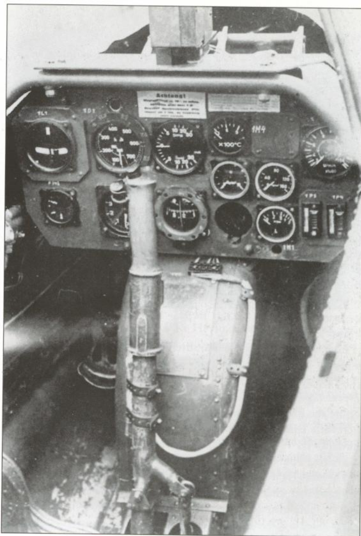
Despite the apparent simplicity of the He 162's instrumentation (flying controls grouped on the left and engine gauges on the right), the Volksjäger was not an easy machine to master. Note the gunsight mounted above the instruments and the rectangular glazed panel (used as a visual retraction check) in the nosewheel housing ahead of the control column
