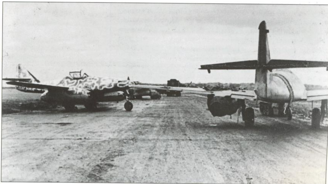
Me 262A-1as of III./KG 54 'Totenkopf' are seen at Neuburg-on-Danube in March 1945. Although no longer fitted with 'Wikingerschiff' weapons pylons beneath the forward fuselage, the spectacularly meander-patterned machine on the left presumably began life as a Jabo model, as it appears to possess only two nose cannon
